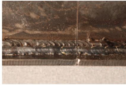
Fig. 5 — Sample of visually acceptable multipass fillet weld with poor fitup and a slugged and bridged root opening that has been welded over as an example. (See Fig. 6.)
